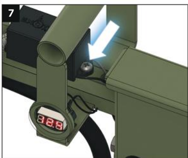
7 Remove the screws holding the HVT (high voltage transformer) to the bar.
