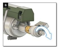
If the nozzle's valve lever is not already positioned on the bottom, we must rotate the pump assembly until it is. Loosen the clamps holding the fuel pump as shown in Step 3.
