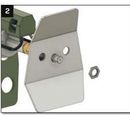
Remove the nut holding the nozzle shield to the nozzle, and move the nozzle shield and electrodes out of the way.
