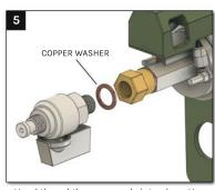
Hand thread the new nozzle into place. Use the 14 mm wrench to keep the check valve from turning while using the adjustable wrench to tighten the nozzle to 80 in-lb.
