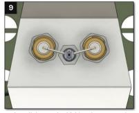
Reinstall the nozzle shield to the new nozzle, and route and install the electrodes. If using a fan type nozzle, be sure the spray is aligned to emit between the electrodes.
