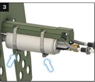
If your electrode wires are tucked, you may need to loosen the clamps holding the fuel pump to make moving things easier. When reinstalling, be sure not to pinch any wires!
