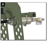
Rotate the pump assembly as necessary and re-tighten all clamps and/or fittings. Fitting (B), if present, must be tightened to 15 ft-lb (180 in-lb), but the pump fitting (C) must be held with a wrench to prevent it from turning.
