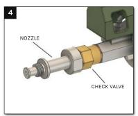
Use a 14 mm wrench to hold the brass check valve in place while using an adjustable wrench to loosen and remove the old nozzle.
