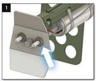
Remove one electrode from the nozzle shield by unscrewing the nut(s) securing it. This will allow easier access for the next step.
