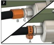
Depending on the type of hose assembly installed, either loosen the hose clamp (A), or loosen the hose end fitting (B) while holding the fuel pump fitting (C) with a 16 mm wrench.
