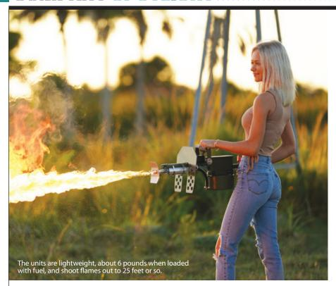
was introduced as the first truly ondemand handheld flamethrower. By using an arc of electricity to ignite the stream of fuel, users don't need to rely on finding pressurized butane canisters and getting a pilot torch running like previous systems on the market. As long as you have power and fuel, you're operational.
